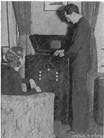
The RCA television receiver. This set employs 30 tubes and is controlled by 14 knobs. Only 70 of these experimental sets were built. When they are placed on the market the number of tubes and knobs will be greatly reduced. These receivers pick up the sound as well as the pictures.
